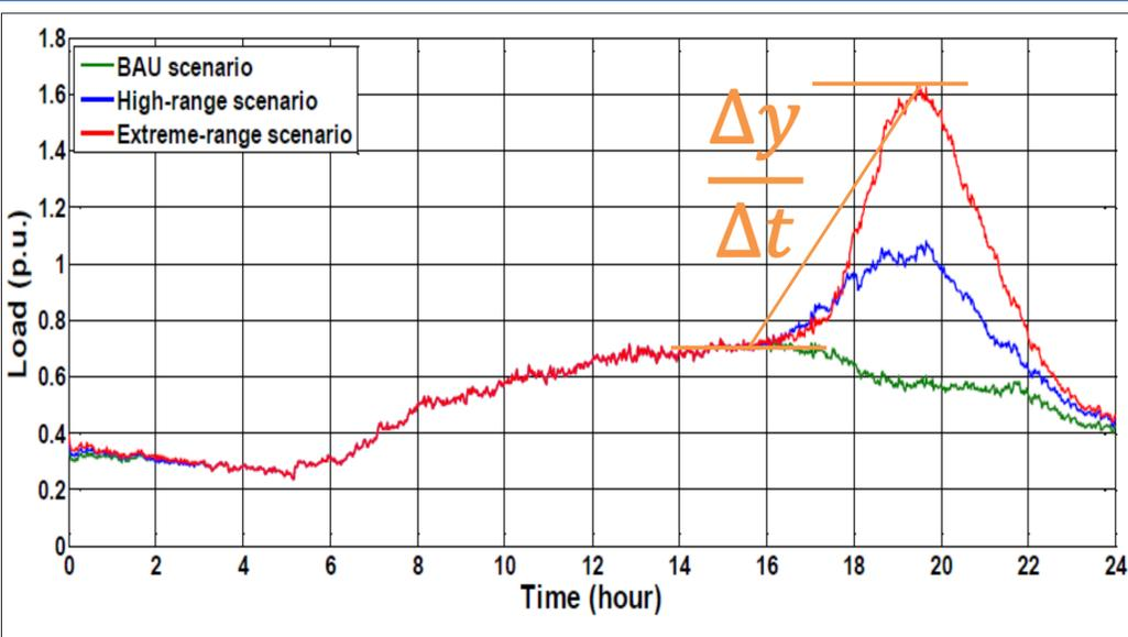
Figure 2 - Load profile showing potential variation in peak load due to electric vehicles [1]
